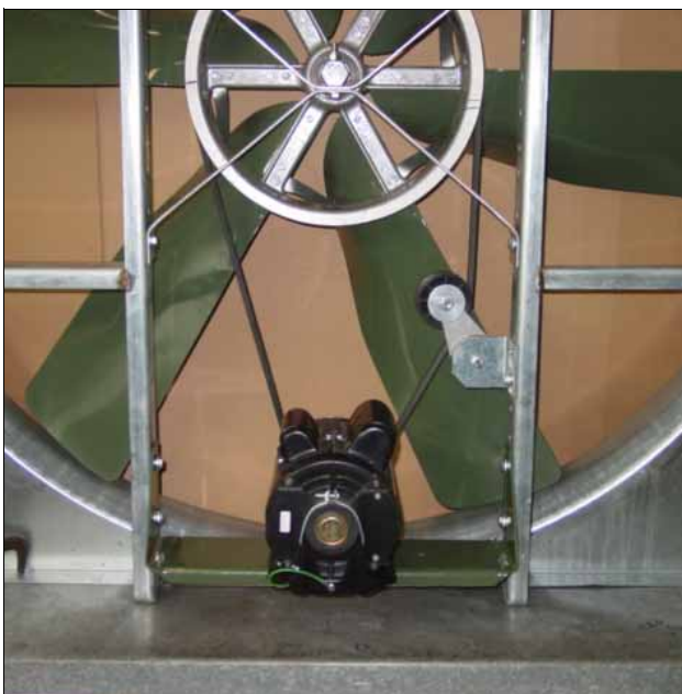
NCF52 with motor mounted at the bottom of the fan
